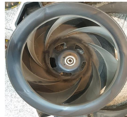
The blowing fan of Cooling & Heating system
